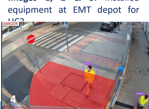
Image 4: Screenshot from camera showing VRU detection and trajectory estimation during technical validation of UC2 at EMT depot.
