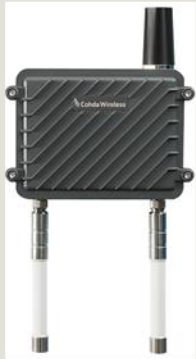
Road Side Unit (RSU)
